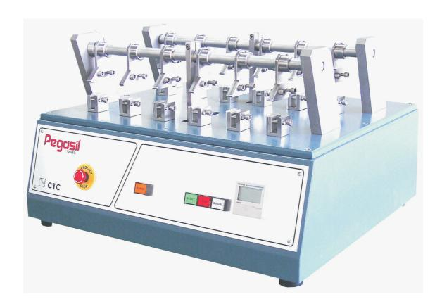
"BALLY" flexing machine with 12 stations
